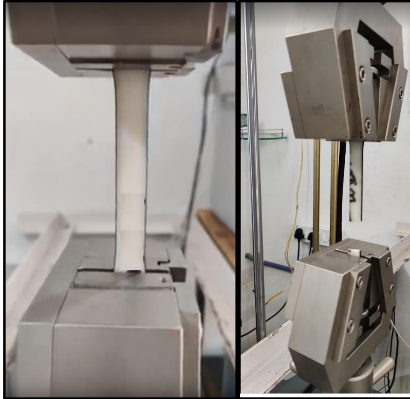
Figure 10: Axial Fatigue Samples under Test at AdvanSES as per ASTM D7791
