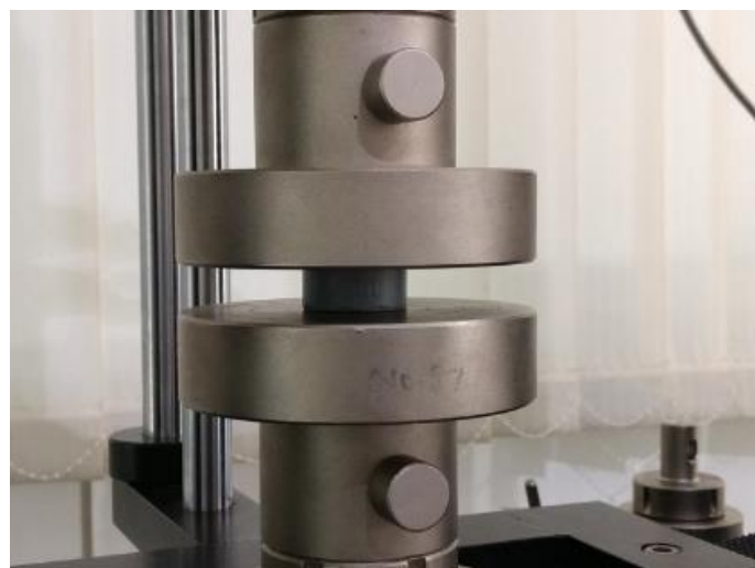
Figure 8: Flatwise Compression Test Setup as per ASTM C365 at AdvanSES
