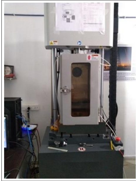
Figure 1.3: AdvanSES High Frequency Testing Setup with Temperature Chamber
