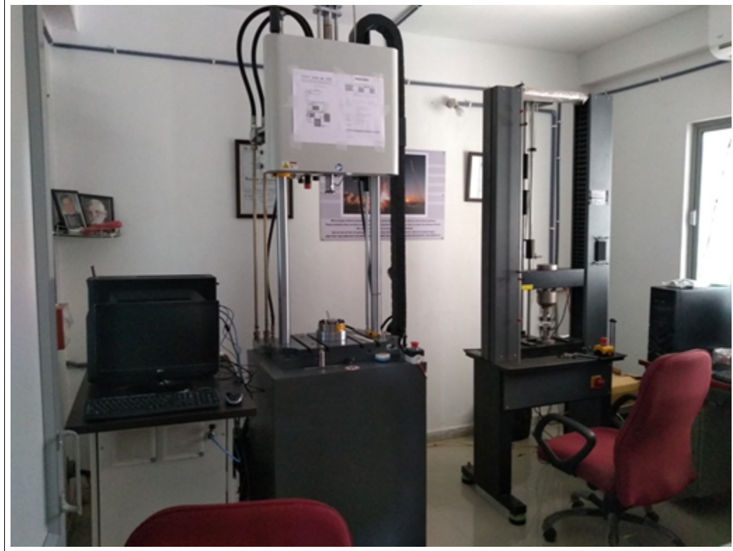
Figure 1.2: AdvanSES High Frequency and ElectroMechanical Testing Setup
