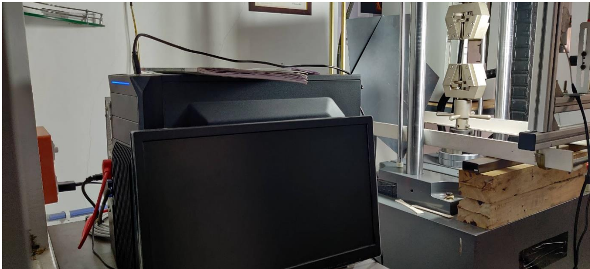
Figure 6: AdvanSES Non-contact Measurement and DIC Setup
